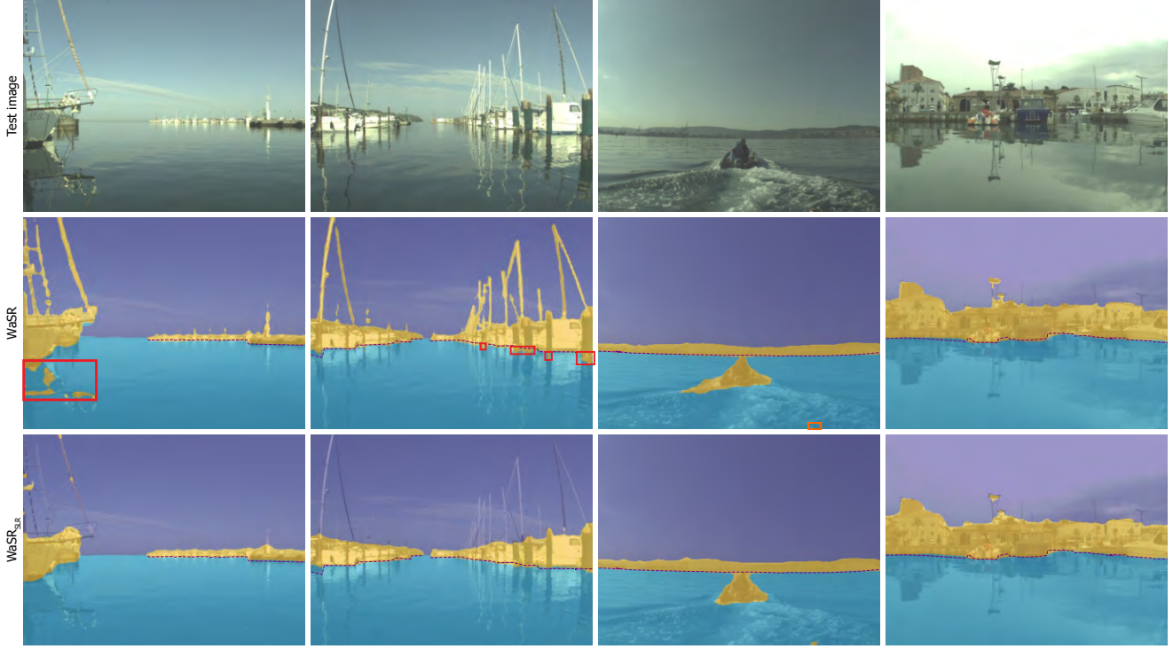
Figure 5: WaSR (fully-supervised) vs. \text{WaSR}_{\text{SLR}} trained using the proposed scaffolding approach. WaSR often predicts false positive detections on water reflections of obstacles (columns 1 and 2), while \text{WaSR}_{\text{SLR}} is more robust. \text{WaSR}_{\text{SLR}} also performs well in difficult scenarios such as wakes (column 3) and heavy reflections (column 4). Best viewed on a screen.
