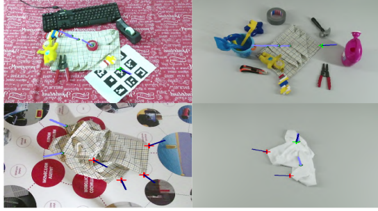
Fig. 4. Examples of false and missed grasp point detections (true as a green cross, false as a red cross, and ground-truth as a green dot).
