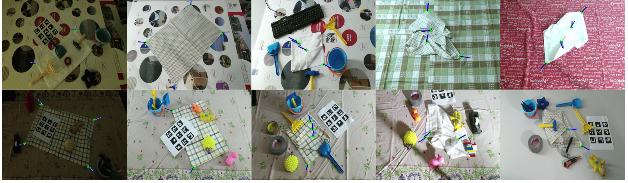
Fig. 3. Several examples of correct grasp point detection (green cross) and estimation of angle-of-approach (dark lines predicted, light lines ground-truth).
