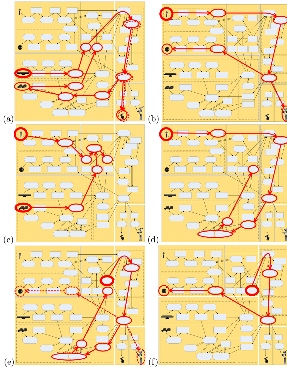
Figure 6. Behaviour mechanisms for components in Figure 5: (a) Attention and exploration mechanisms. (b) Answering tutor's requests. (c) Merging multi-modal information. (d) Situated tutor-driven learning. (e) Situated autonomous and tutor-assisted learning. (f) Non-situated tutor-assisted learning.
