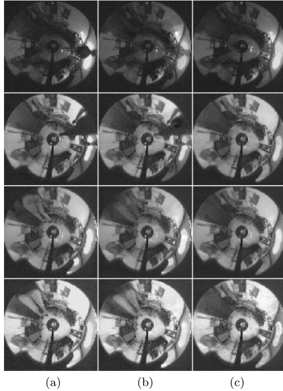
Fig. 4. (a) Four panoramic images from the sequence, (b) their reconstructions based on the standard PCA, and (c) their reconstructions based on the robust PCA.
