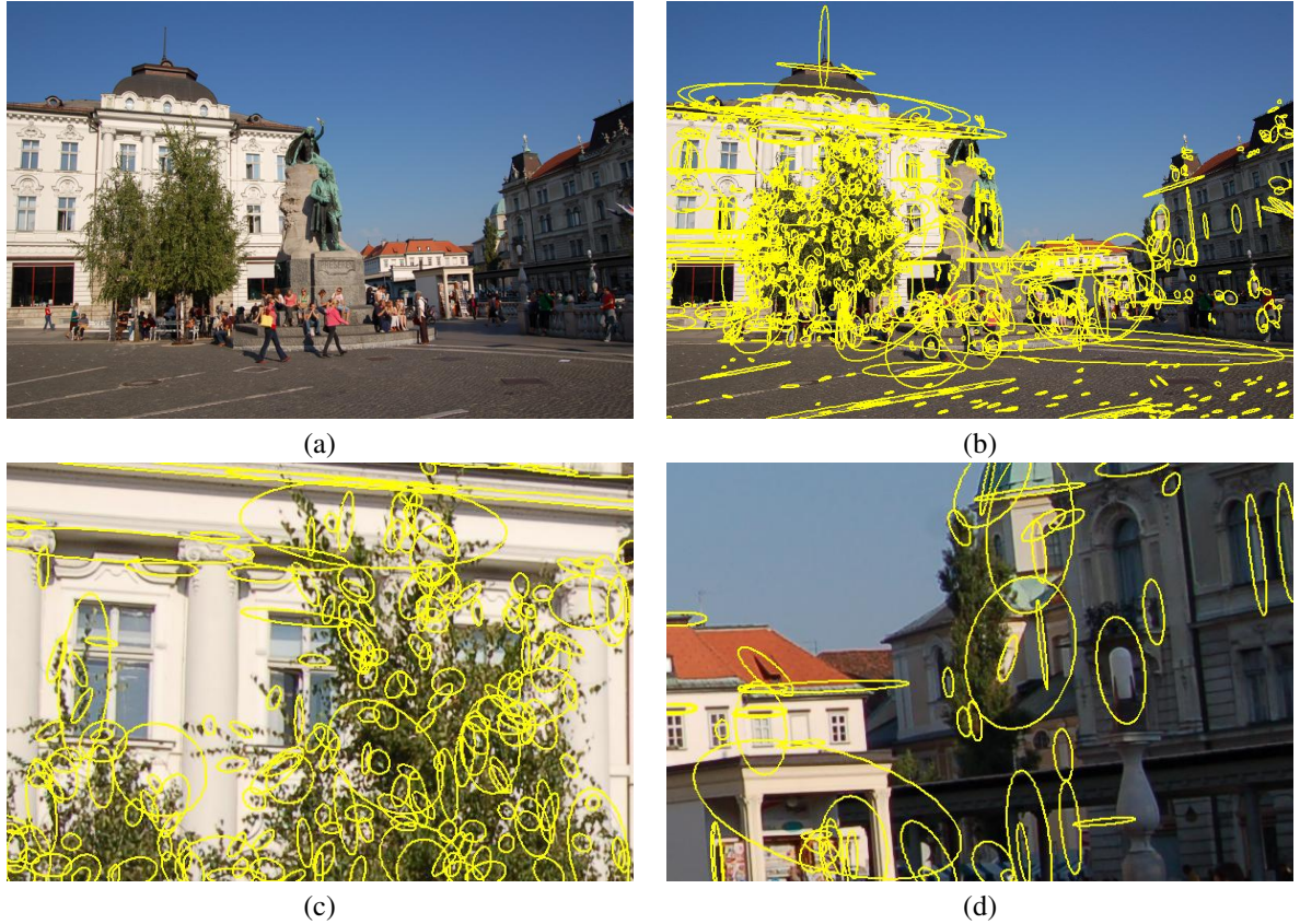
Figure 1: Vegetation segmentation for boosting performance of MSER feature detector: (a) Input image and (b) the detected MSER features (depicted as ellipses fitted to the detected maximally stable extremal regions). Please note, that out of 5195 detected MSER features, 2130 are located on vegetation. In (c) and (d) two image sections of the same size are shown. The section in (c) includes lots of vegetation and within this section 777 MSER features are detected. The section in (d) includes much less vegetation and within this section only 200 features are detected. For clarity sake, only every fourth MSER feature is shown.
