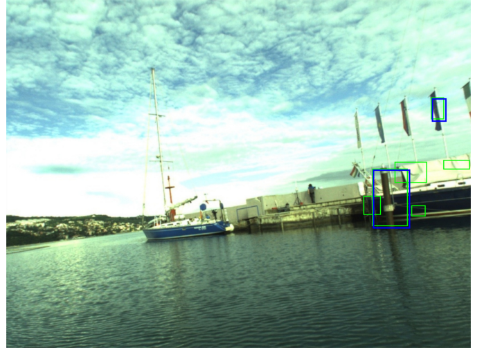
Fig. 8. Obstacle detections before and after affinity propagation clustering. Initial detections are shown in green, while the clustered detections are represented in blue.
