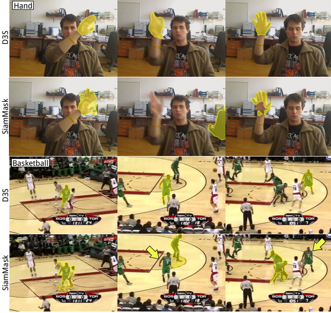
Fig. 13. D3S 2 vs. SiamMask segmentation quality. Hand : the rigid template in SiamMask fails on a deforming target, the GIM model in D3S 2 successfully tracks despite a significant deformation. Basketball : SiamMask drifts to a similar object, while D3S 2 leverages the discriminative learning in GEM to robustly track the selected target. The yellow arrow denotes the target which should be tracked.
