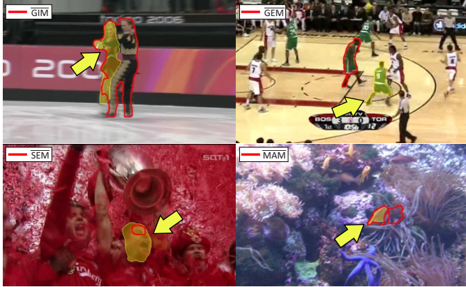
Fig. 12. Tracking results of D3S 2 (yellow mask) compared to D3S 2 variations (red) with the individual modules, GIM, GEM, SEM and MAM, removed. The arrow indicates the tracked target.
