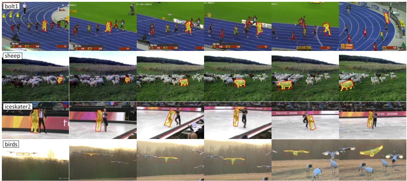
Figure 7. Sequences with distractors (similar objects in the target vicinity). D3S segments the correct target even though a similar target is close (or even overlapping). These examples show discriminative power of the proposed tracker achieved by the discriminative GIM and GEM.
