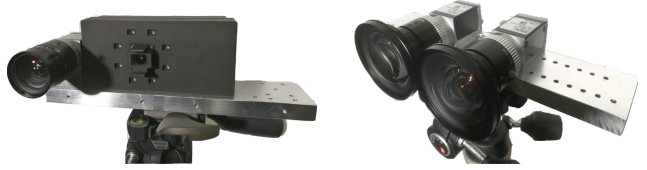
Figure 2. Two of the three sensors used in dataset acquisition: ToF-RGB-pair (left) and a stereo-camera pair (right). The third sensor, Kinect v2, is standard.
