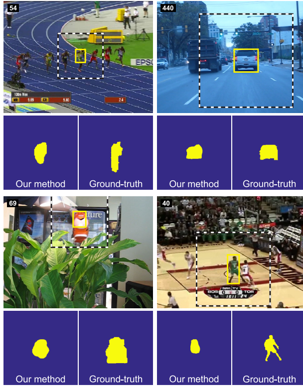
Figure 10: Qualitative comparison of the spatial reliability maps during tracking. The dashed bounding box represents area from which correlation filter is obtained. This is also the area where spatial reliability map is calculated. In addition, the ground-truth segmentation masks are visualized on the right side under each frame.
