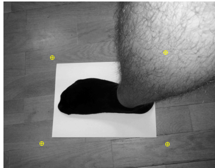
Figure 3.1: Input image I with coarse reference object location estimation, marked by yellow circles with plus signs.
