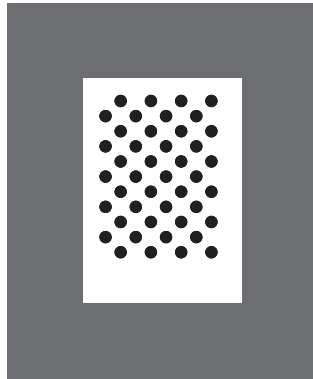
Figure 5.1: The calibration board, with an A4-sized rectangle, a 10 cm dark gray margin and a calibration pattern.
