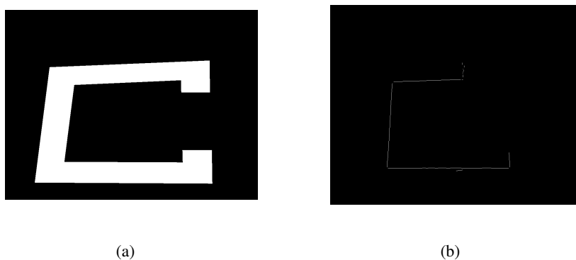
Figure 3.7: Figure 3.7a shows the Region of interest mask ROI , whereas Figure 3.7b shows the Final edge image E' , obtained by applying the ROI mask to E .
