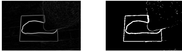
Figure 3.3: Gradient magnitude image G of the input image (left), and the mask M (right) obtained from thresholding G .
