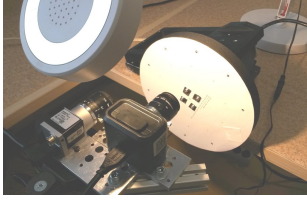
Figure 1: The experimental scene setup with strong lighting. The frame-based Basler (left) and the event-based ATIS (right) cameras are watching the white rotating disk with nine ArUco markers. A nonflickering LED lamp illuminates the scene from the top.
